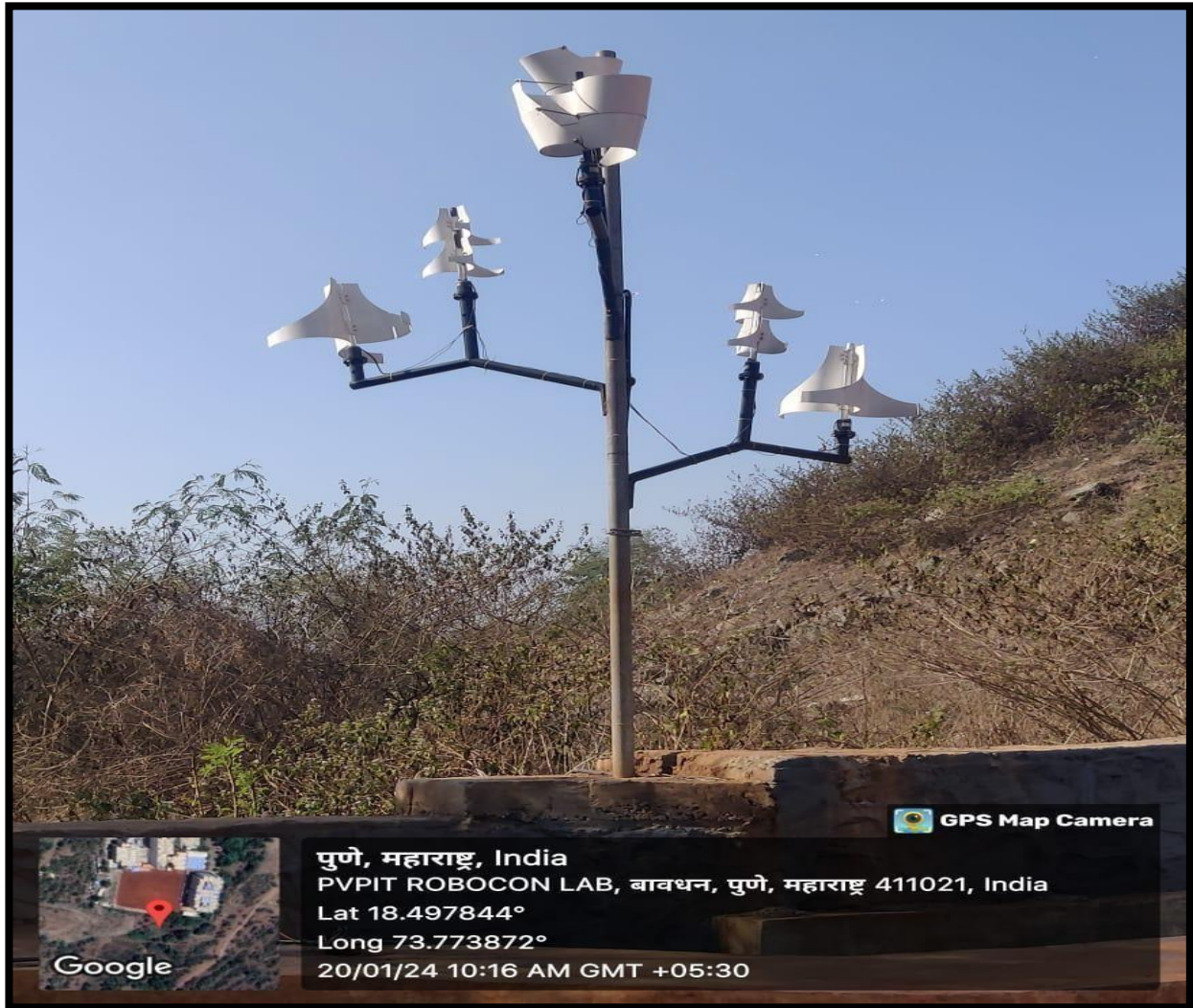
Parametric Evaluation of Vertical Wind Tree with 3 branches and 6 turbines installed at PVPIT ground
